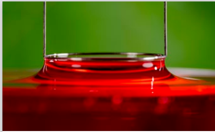
Du Noüy ring with liquid lamella
