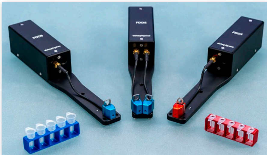
Fig. 1: The FDDS FlexDrop dosing system is available in three variants. The FDDS Nano and FDDS Double Nano can dose one or two liquid drops with a minimum volume of 2 nL and the FDDS Pico can dose one liquid drop with a minimum volume of 25 pL.
