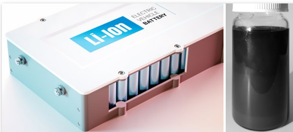
Fig. 1 left: Battery pack for electric vehicle right: Battery slurry 1 in sample container after 26 hours
