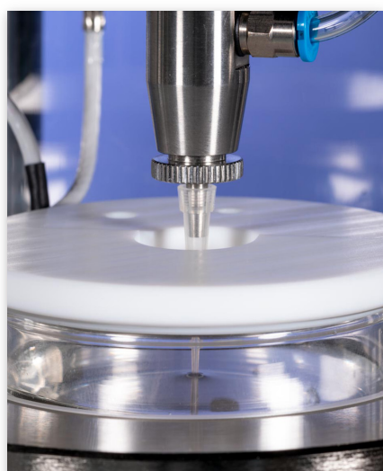
Fig. 3: Disposable capillaries attached in MBP 200 with PTFE cover
