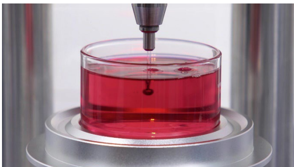
Figure 2: When using the maximum bubble pressure method, gas bubbles are generated in the liquid to be examined via a capillary.
