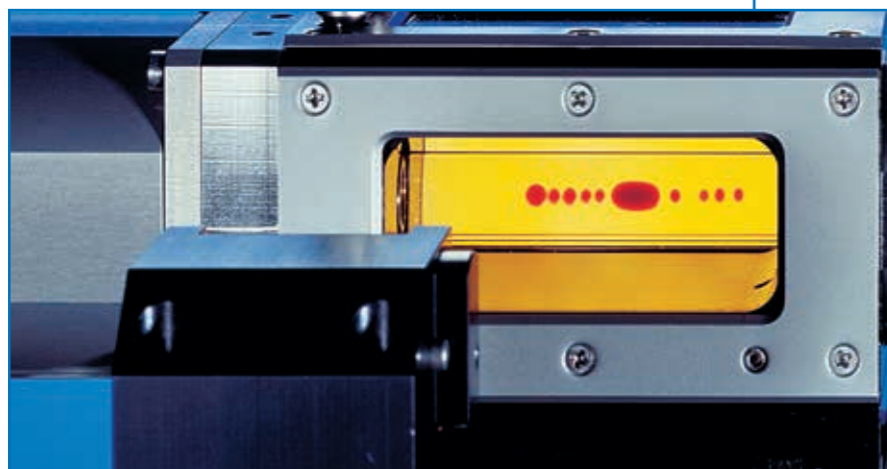
Spinning drops in SVT 15N capillary
