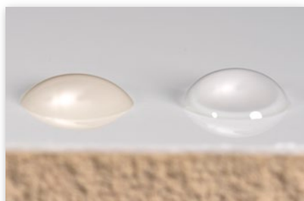
The contact angles of two test liquids serve as the basis for calculating the surface energy of the solid surface.
