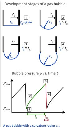
A gas bubble with a curvature radius  $r_{\rm B}$ , suspended at the capillary opening with the inner radius  $r_{\rm C}$ , goes through several stages of development. At the time of maximum bubble pressure  $\exists$ , the dynamic surface tension can be determined.
