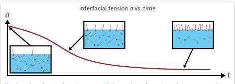
The dynamic surface tension  $\sigma$  decreases with time as the surface-active substances accumulate at the surface. The static surface tension is established after the equilibrium is reached.
