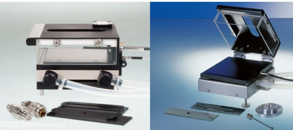
The formation of ice on **airplane wings** influences the aerodynamic properties and the stability of the aircraft. In order to guarantee highest levels of comfort and safety, even at freezing cold temperatures, **de-icing fluids** are used extensively. Their wetting behaviour can be investigated at temperatures of down to -30 °C in a suitable environmental chamber from DataPhysics Instruments.
