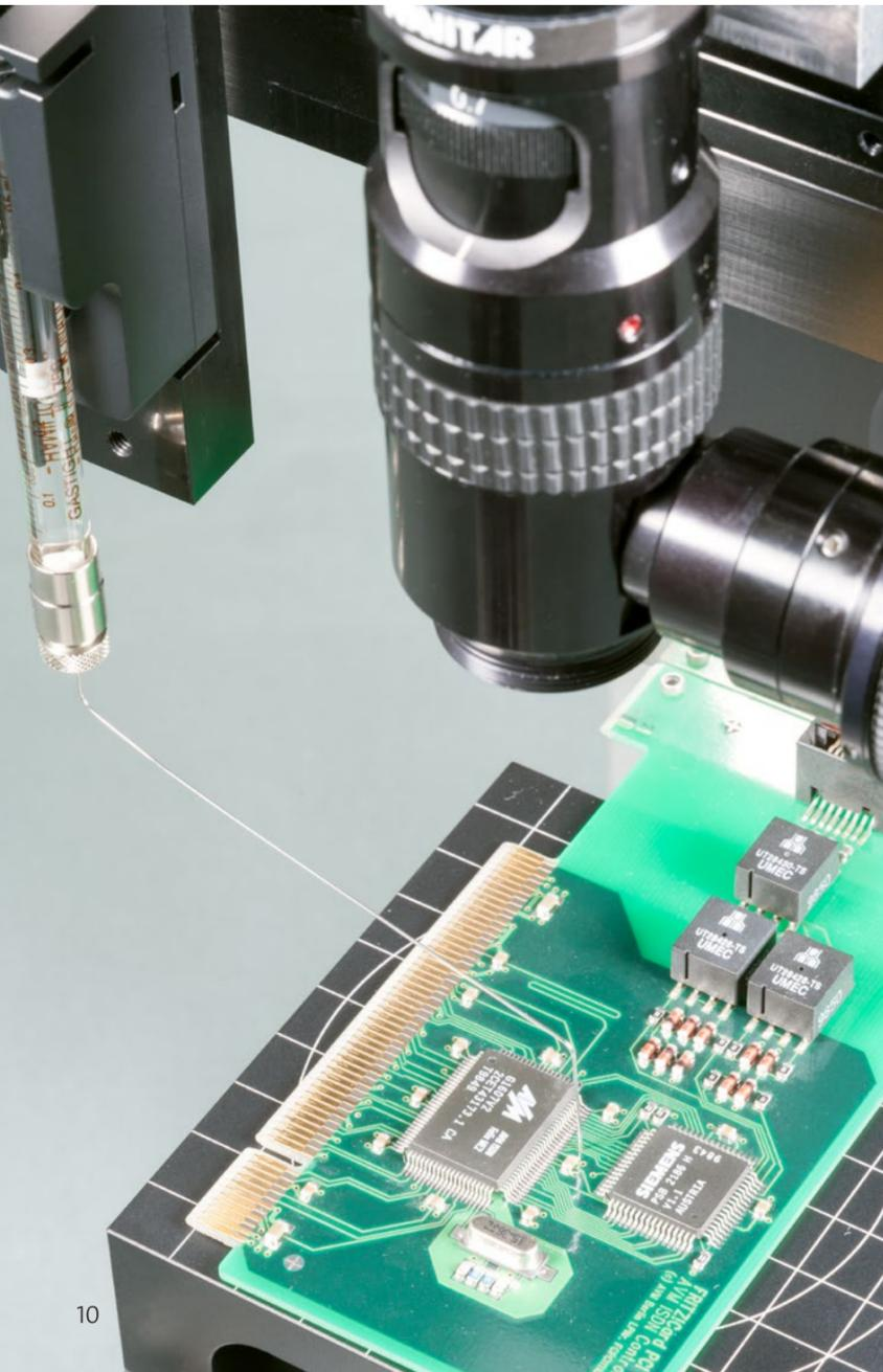
The **Topview Video System TVS** opens up a completely new approach to contact angle measurement. With this system deposited drops are monitored and evaluated in **topview** which allows to investigate previously inaccessible sample spots. Exclusively with the TVS contact angles can be measured, for example, at the bottom of indents of ready-made components or on assembled printed circuit boards. Moreover, the TVS enables the determination of **surface homogeneity** and **surface isotropy**.
