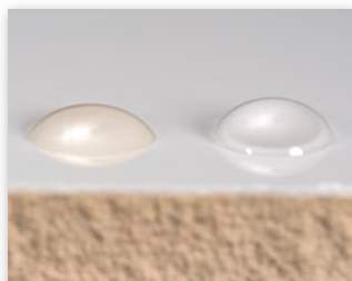
Two test liquids are used to determine the surface energy.
