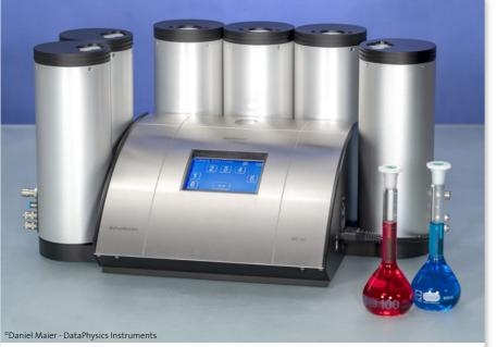
The MultiScan MS 20 dispersion stability analysis system from DataPhysics Instruments can be equipped with six independent sample chambers, called ScanTowers.
