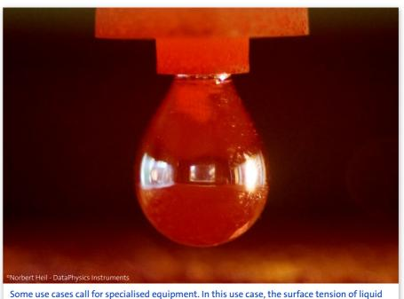
Some use cases call for specialised equipment. In this use case, the surface aluminium was measured at 700  $^\circ \rm C.$
