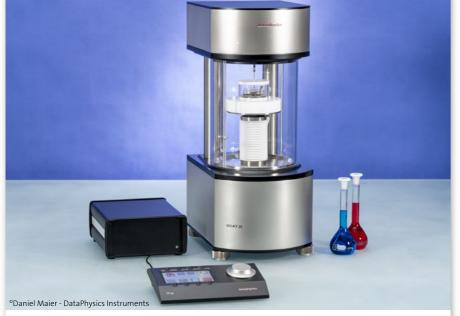
The tensiometers of the DCAT series can calculate contact angles even for extremely hydrophilic surfaces, such as the screw threads of dental implants.
