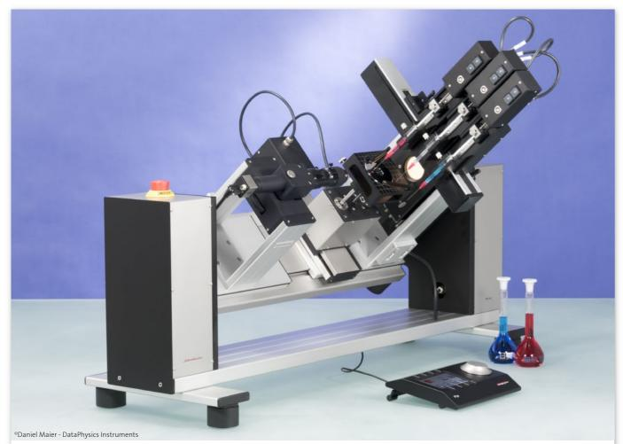
Measurement equipment can be individually assembled to fit a specific use case. For example, using the TBU tilting base unit, a sessile drop can be tilted to measure the drop's receding and advancing contact angle.
