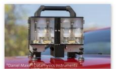
The PCA 100 portable contact angle measuring system is groundbreaking in its design. It enables "on-the-go" contact angle measurements, even on large surface areas.
