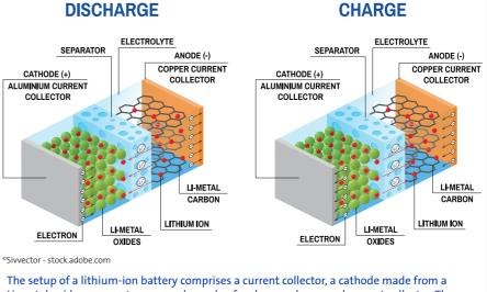
Li-metal oxide, a separator, an anode made of carbon, and a second current collector. The cathode, anode, and separator are submerged in an electrolyte.
