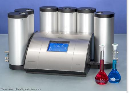
The MultiScan MS 20 dispersion stability analysis system from DataPhysics Instruments can be equipped with six independent sample chambers, called ScanTowers.
