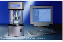
The force-based tensiometers of the DCAT series is the first major enhancement to the portfolio of DataPhysics Instruments. With standard test methods such as the Du Noüy ring method and advanced evaluation capabilities, such as dynamic contact angle measurements, the new devices further strengthen the company's position as a competent and valuable partner for surface and interfacial science applications.
