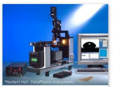
The OCA 40Micro with a nanolitre or picolitre dosing system enables contact angle measurements on the smallest structures.
