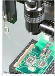
With the TVS Topview Video System, contact angle measurements in indentations are possible.
