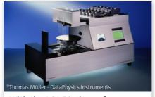
With the ACA 50, the surface energy of, for example, a silicon wafer can be determined fully automatically within a compact instrument design.
