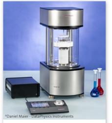
With a DCAT tensiometer, the surface tension of an electrolyte solution can be easily determined. Together with a Peltier temperature control unit, the sample vessel can be tempered from -15 to 135 °C.
