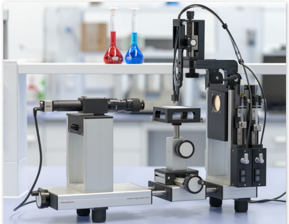
Fig. 1: DataPhysics Instruments OCA 25 with Double Liquid Jet system DLJ
