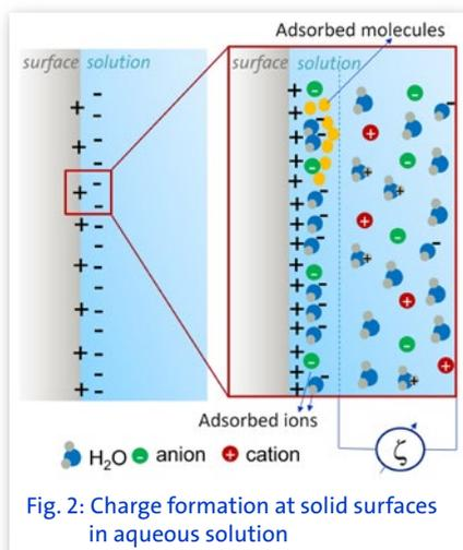
Fig. 2: Charge formation at solid surfaces in aqueous solution
