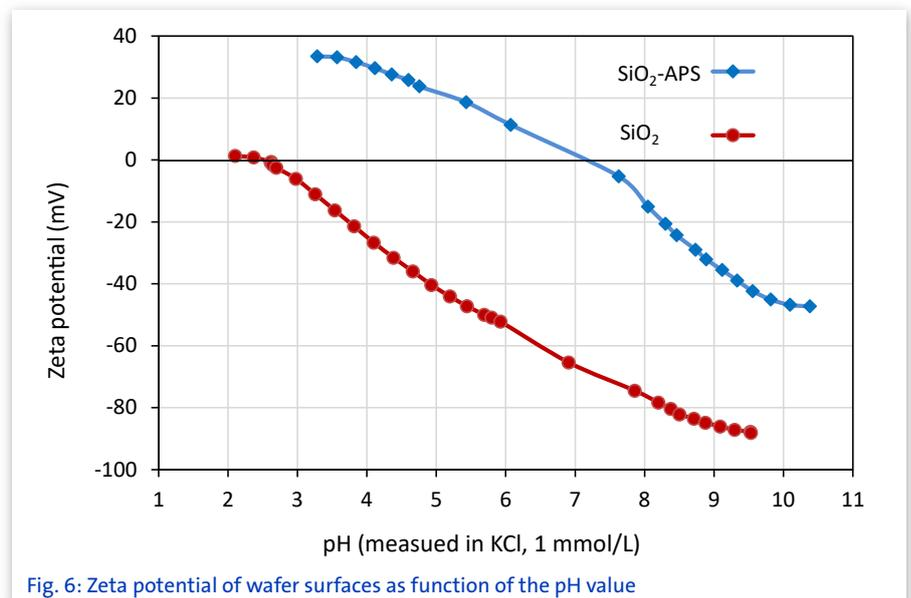
Fig. 6: Zeta potential of wafer surfaces as function of the pH value
