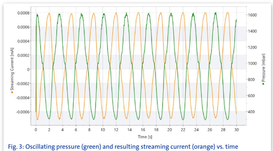
Fig. 3: Oscillating pressure (green) and resulting streaming current (orange) vs. time
