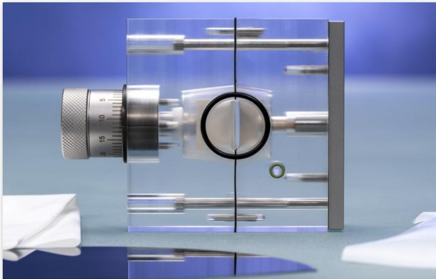
Fig. 4: The MC-ZPA/S measuring cell enables measurements of zeta potential of plate shaped solids, such as wafers or plastic sheets.
