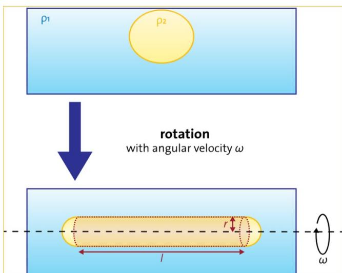
Fig. 2. Drop deformation with the spinning drop principle
