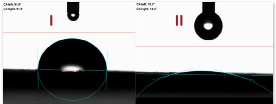
Fig. 5: Initial water drop (I) and final water drop (II) on sample C.
