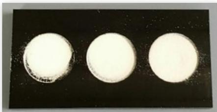
Fig. 3: The sample container for powders ST-P.
