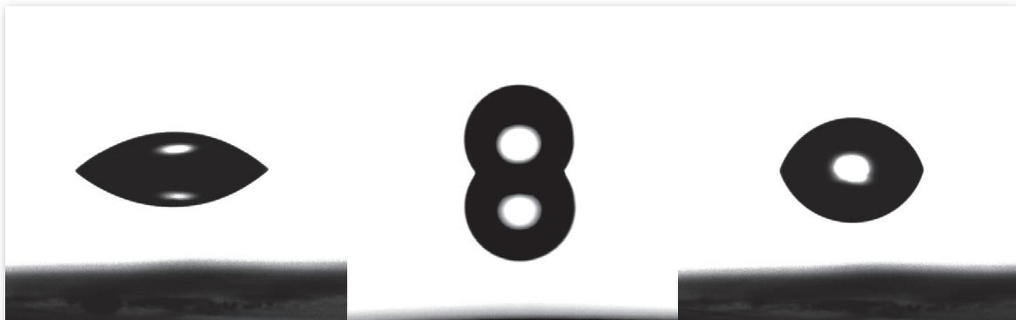
A contact angle of approximately  $40^\circ$  is formed on untreated platinum (left). The platinum surface coated with SAMs out of a solution forms a contact angle of  $126^\circ$  (centre). The platinum surface coated with SAMs out of the vapour phase shows an angle of  $72^\circ$  (right).
