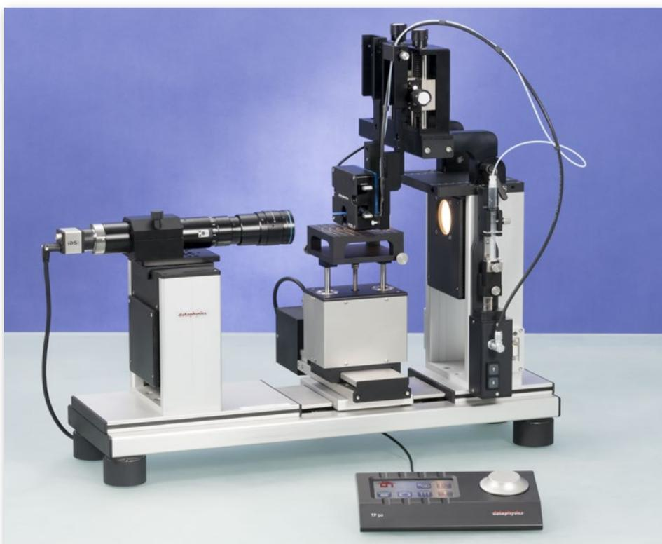
The OCA 200 contact angle meter from DataPhysics Instruments was specially developed to measure on the smallest surface areas.
