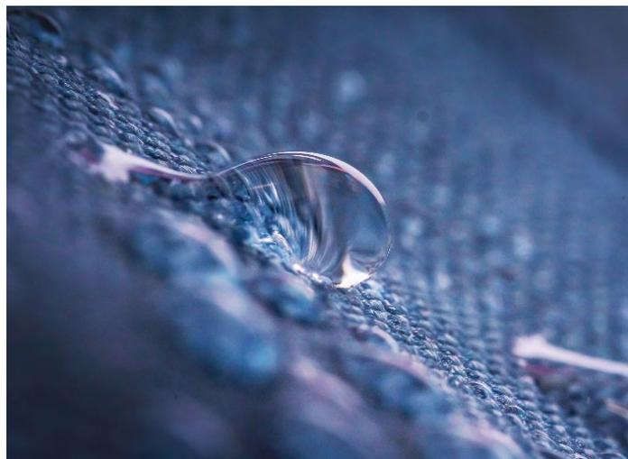
Fig. 1. Water droplet rolling off a hydrophobic surface.
