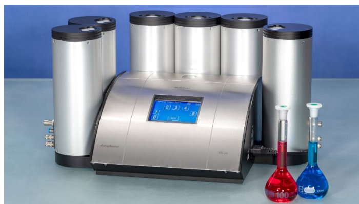
Fig. 2. DataPhysics Instruments stability analysis system MultiScan MS 20 with six independent Scan Towers.
