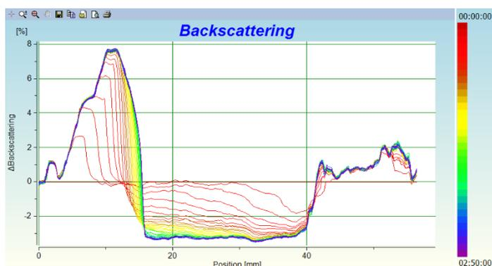
Fig. 4. Backscattering intensity diagram of seasoning oil 1
