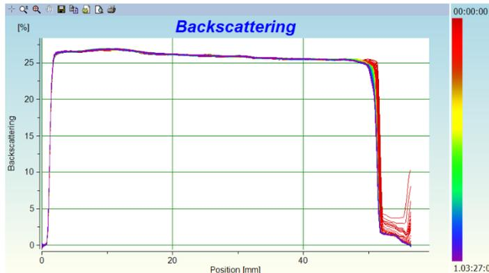
Fig. 4: Backscattering intensity diagram of ink 1.
