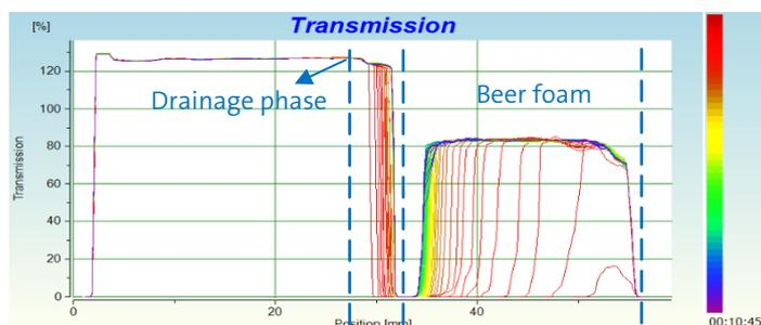
Fig. 4: Transmission intensity diagram of light beer.
