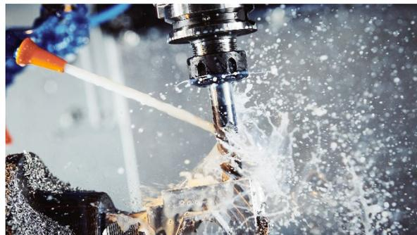
Fig. 1. Cutting fluid in metalworking processes.
