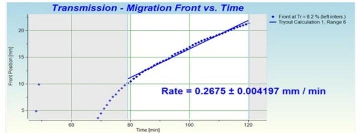
Fig. 7. Migration front analysis (between 79 min and 120 min) of the phase separation taking place during the first experiment.
