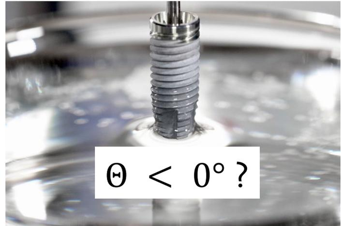
Fig. 1. The surface of dental implants is very hydrophilic. Thus, water spreads on it, which conventionally means the contact angle is  $0^\circ$ . However, imaginary contact angles allow further discrimination...
