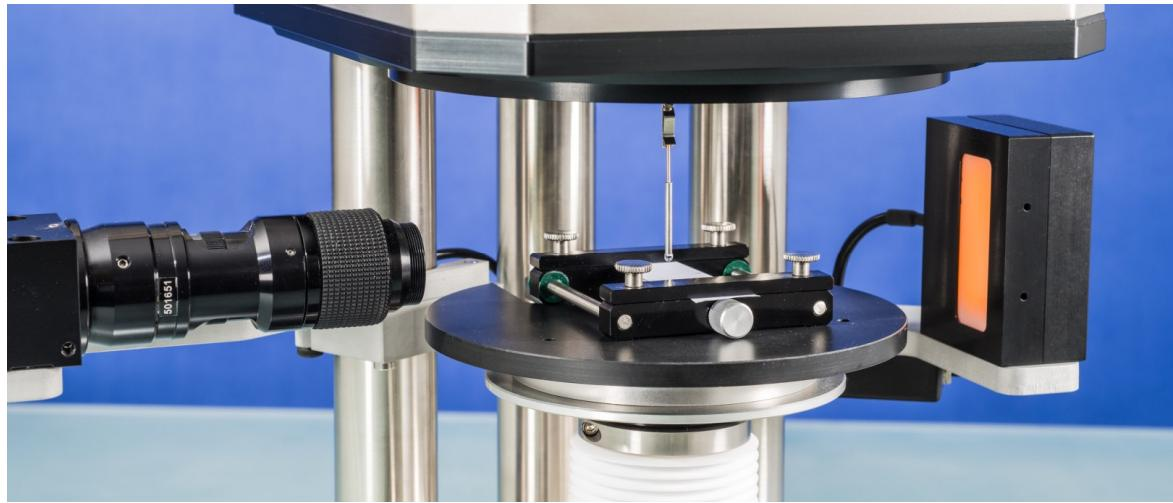
This system combines a force measurement to determine the force of adhesion and an optical system to determine the area of contact between the liquid/gas and solid phase for each force that is measured. Like this a force per area can be determined. The measurement procedure involves a liquid or gas bubble being pushed onto a solid substrate under air or liquid and being pulled off from it again.
