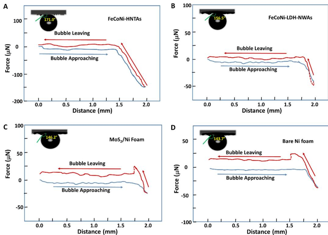
**Figure 2.** Adhesive force and contact angle measurements of gas bubbles on FeCoNi-HNTAs, FeCoNi-LDH-NWAs, MoS<sub>2</sub>/Ni Foam, and bare Ni foam.
