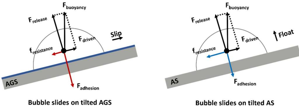
**Picture 3:** Force analysis of the bubbles on AGS and AS
