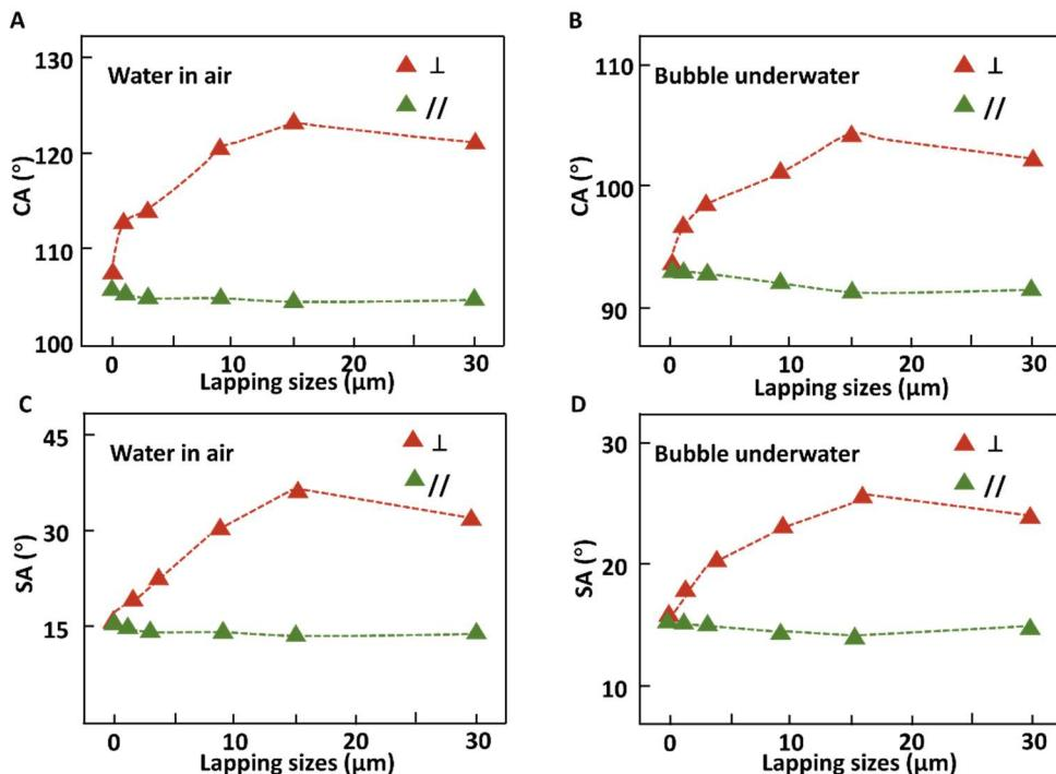
**Picture 2:** CAs changes on AGSs with increasing lapping size, for 5  $\mu$ L water droplets in air (A) and 5  $\mu$ L air bubbles underwater (B). SAs changes on the AGSs with increasing lapping size, for (C) 5  $\mu$ L water droplets in air and (D) 5  $\mu$ L air bubbles underwater
