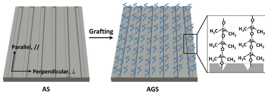
**Picture 1:** Preparation of anisotropic covalently grafted slippery surfaces AGSs by grafting PDMS on anisotropic surfaces (ASs)
