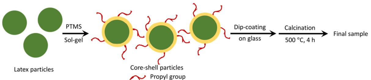
**Figure 1:** Preparation process of superhydrophilic antireflective coatings
