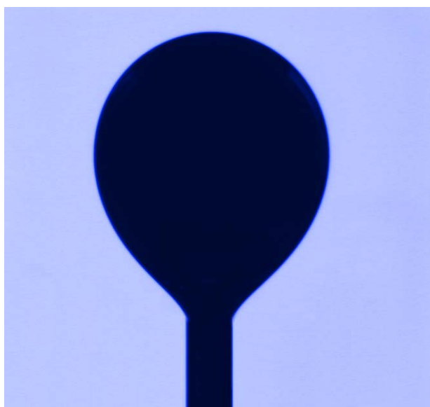
Diagram 1: Image of a paint drop in Perfluorohexane
