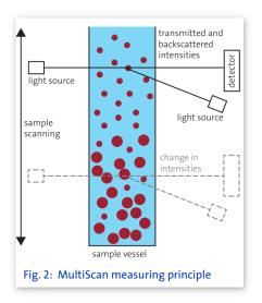
the detector, for measuring the backscattered light (Fig. 2). The light sources and detector move up and down along the sample vessel for each measurement so that position-resolved light intensities can be recorded. So far, ScanTowers utilizing infrared LEDs (i.e. IR tower) have been widely used for dispersion stability analysis.
